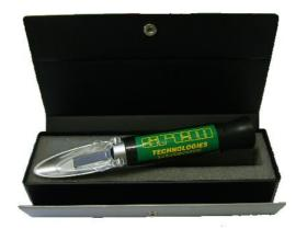
The hand-held refractometer is a simple device to control the concentration of emulsifier.
